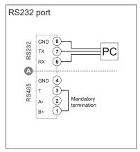
**NOTE.** RS485: additional devices provided with RS485 are connected in parallel. The termination of the serial output is carried out only on the last instrument of the network, by means of a jumper between (B+) and (T). The communication RS232 and RS485 ports **can't be** connected and used simultaneously.
