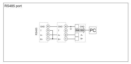
**NOTE.** RS485: additional devices provided with RS485 are connected in parallel. The termination of the serial output is carried out only on the last instrument of the network, by means of a jumper between (B+) and (T).
