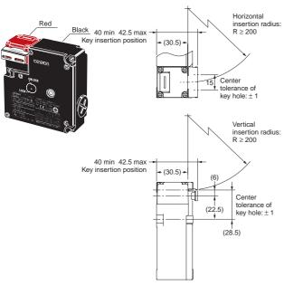
D4NL + D4DS-K2 (with Top-inserted Operation Key)
