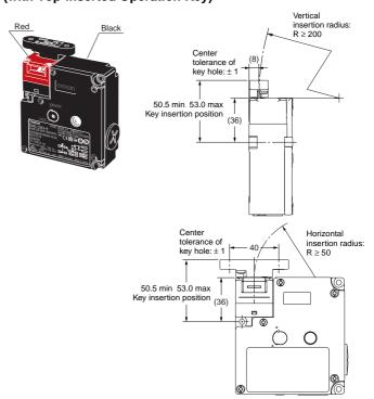
D4NL + D4DS-K5 (with Front-inserted Operation Key)
