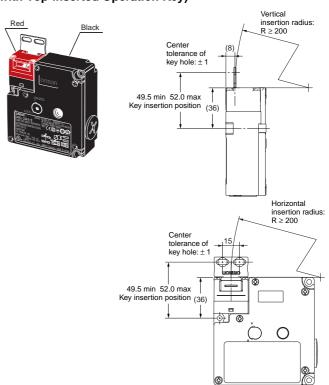
D4NL + D4DS-K2 (with Front-inserted Operation Key)
