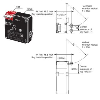
D4NL + D4DS-K1 (with Top-inserted Operation Key)
