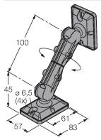
7030296 Arm bracket for UHF RFID read/write heads TNxxx-Q175L200-H1147, TNxxx-Q240L280-H1147 and TNxxx-
