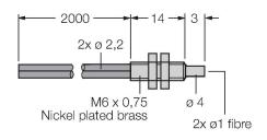
Plastic fiber-optic sensor, operating mode: Diffuse mode, threaded sleeve M3 x 0.75 mm, field wireable wire without end tip, polyethylene sheath, ambient temperatures -30 °C...+70 °C
