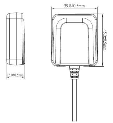
The dimension of GR-701 is 40 mm (W) x 45 mm (L) x 16 mm (H) as shown above.
