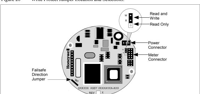
Figure 20 Write Protect Jumper Location and Selections.
