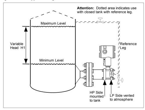
Figure 10 Typical Flange Mounted Transmitter Installation
