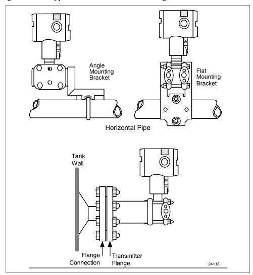
Figure 8 Typical Bracket Mounted and Flange Mounted Installations
