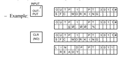
• Be sure to store all changes in the transmitters non-volatile memory by pressing the [SHIFT] key and then the [ENTER] key.
