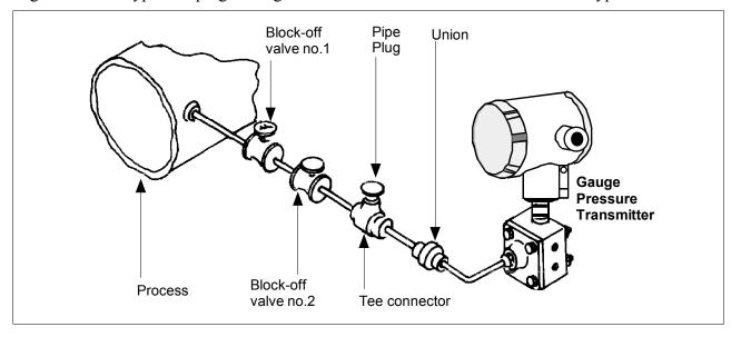
Figure 44 Typical Piping Arrangement for Liquid Level Measurement with GP Type Transmitter
