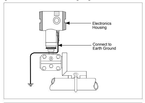
Figure 18 Ground Connection for Lightning Protection.
