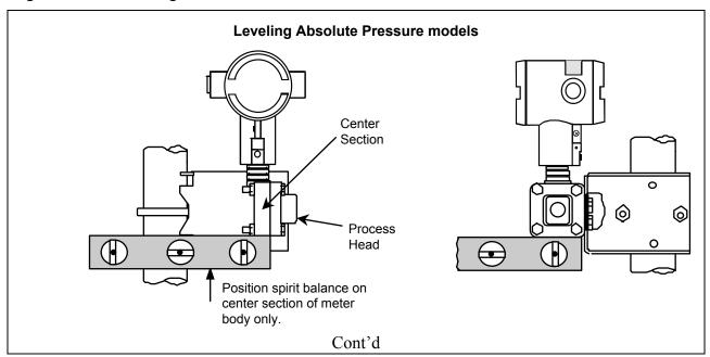
Figure 9 Leveling an Absolute Pressure Transmitter (cont'd)
