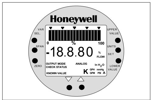
Please refer to Table 31 in this manual for a description of the pushbuttons on the meter face. See Section 8.6 for a description of the indicators with examples of typical display indications and error codes. (Note that the display may revert to dashes (---) after the self-test until the transmitter initializes all its functions.) Use the SFC to check the transmitter's status.
