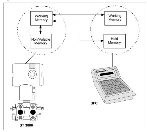
Figure 24 SFC and ST 3000 Transmitter Memories.
