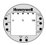
New Smart Meter with Local Zero and Span New Smart Meter Connections – The new integral smart meter (8-wires) is connected directly to the transmitter's PWA and is mounted to the electronics module assembly inside the electronics housing. The new integral smart meter is designed for the ST 3000 Release 300 transmitter and provides functionality not available with other smart meter designs.
