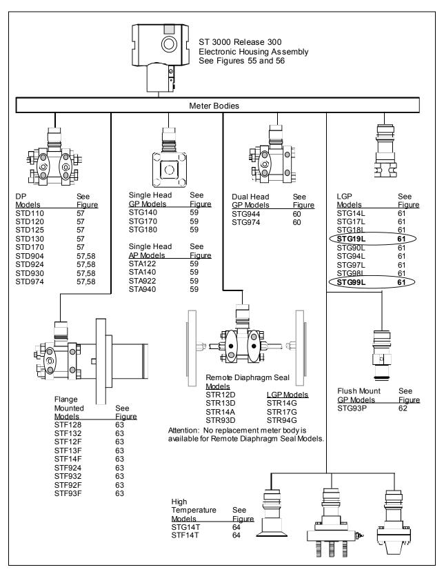
Figure 53 Major ST 3000 Smart Transmitter Parts Reference.
