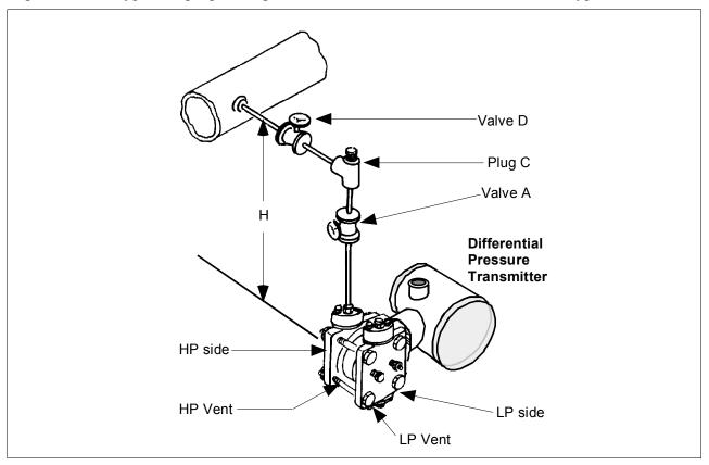
Table 40 Starting Up DP Transmitter for Pressure Measurement With SFC
