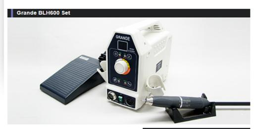
Your Brush motor hand piece and Brushless motor hand piece can be alternately used in one controller because of **New Hybrid system** which is adopted for this Hybrid Micromotor system GRANDE set. As further attractive functions, you can experience the **Auto-cruise system** which the hand piece is run at the same rotation speed even if you step out from the foot pedal.
