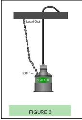
In some applications it may not be possible to install the transducer using either a flange or the 1" BSP thread, in these circumstances it may be possible to suspend the transducer from its cable. In these installations it is recommended that the transducer be secured using a small chain fitted to one of the chain holes on the top of the transducer, see figure 3.
