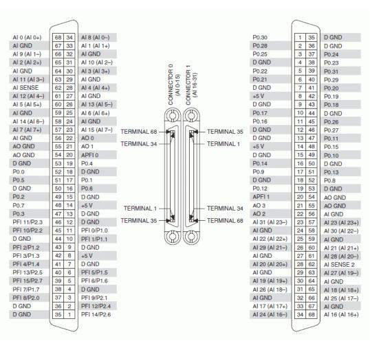
NI PCIe/PXIe-6363 Pinout
