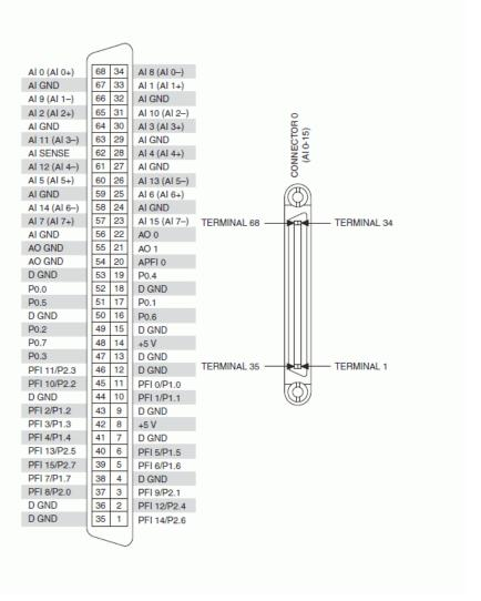
NI PCIe/PXIe-6361 Pinout
