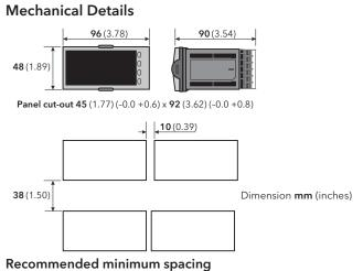
If more than one unit is mounted in the same panel they should be spaced to allow sufficient air flow between them.
