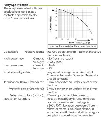
above. Absolute max switching capability: <2A at 240V RMS (resistive loads)
