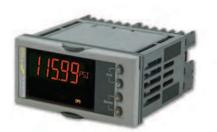
Model number 32h8e is a horizontal 1/8DIN indicator and alarm unit that performs the dual function of remote display for EPower and independent 'policeman'. The latter is intended to disconnect should an overtemperature (or other excess process condition) occur.
