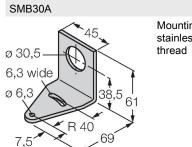
Mounting bracket, rectangular, stainless steel, for sensors with 30mm thread
