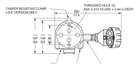
ZERO ADJUSTMENT SCREW ALLOW 150 mm (6.0 in) CLEARANCE FOR ZERO ADJUSTMENT
