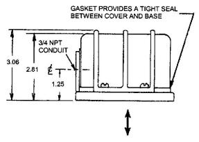
DIRECTION OF SENSITIVITY TO VIBRATION (PEAK ACCELERATION)
