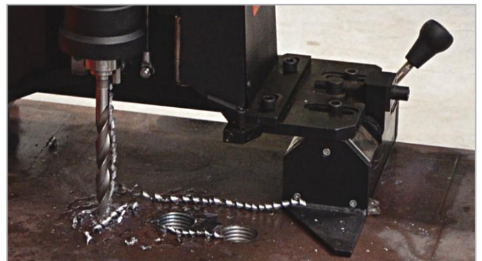
Clamping base incorporates cross slide system for precise hole center locations. Both 44 mm longitudinal and cross travel.
