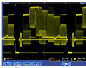
Viewing an NTSC video signal. Notice the intensity-graded view provided by the DPO's ability to represent time, amplitude, and distribution of amplitude over time.
