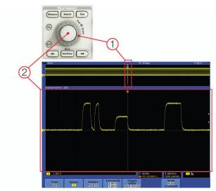
Wave Inspector controls provide unprecedented efficiency in viewing, navigating, and analyzing waveform data. Zip through your 10M point record by turning the outer pan control (1). Get from the beginning to end in seconds. See something of interest and want to see more details? Just turn the inner zoom control (2).
