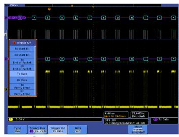
Capture – Triggering on a specific transmit data packet going across an RS-232 bus. A complete set of triggers, including triggers for specific serial packet content, ensures you quickly capture your event of interest.
