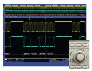
Search - I2C decode showing results from a Wave Inspector search for Address value 50. Wave Inspector controls provide unprecedented efficiency in viewing and navigating waveform data.
