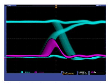
Digital phosphor technology enables greater than 50,000 wfm/s waveform capture rate and real-time intensity grading on the MSO/DPO4000 Series.
